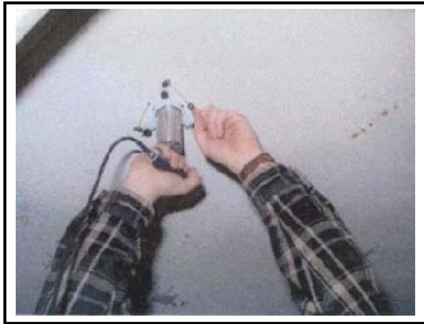
Figure 6:9-2: Inspector Using an Impact Echo Test Unit
