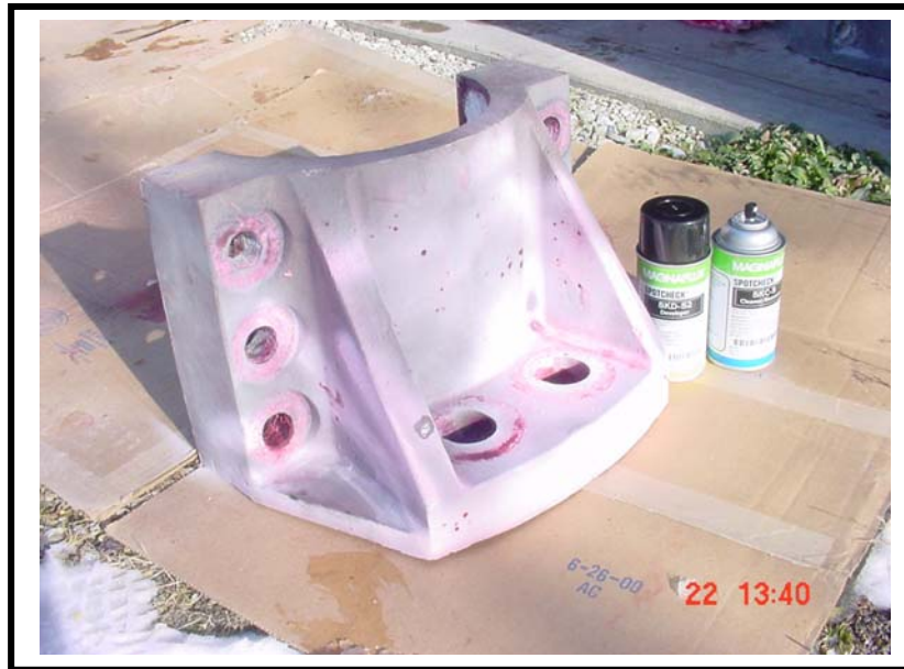
Figure 6:15-1: Visible Dye Penetrant and Developer Applied to a Casting
