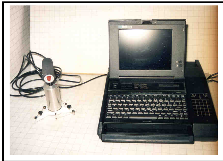
Figure 6:9-1: Impact Echo Test Unit
