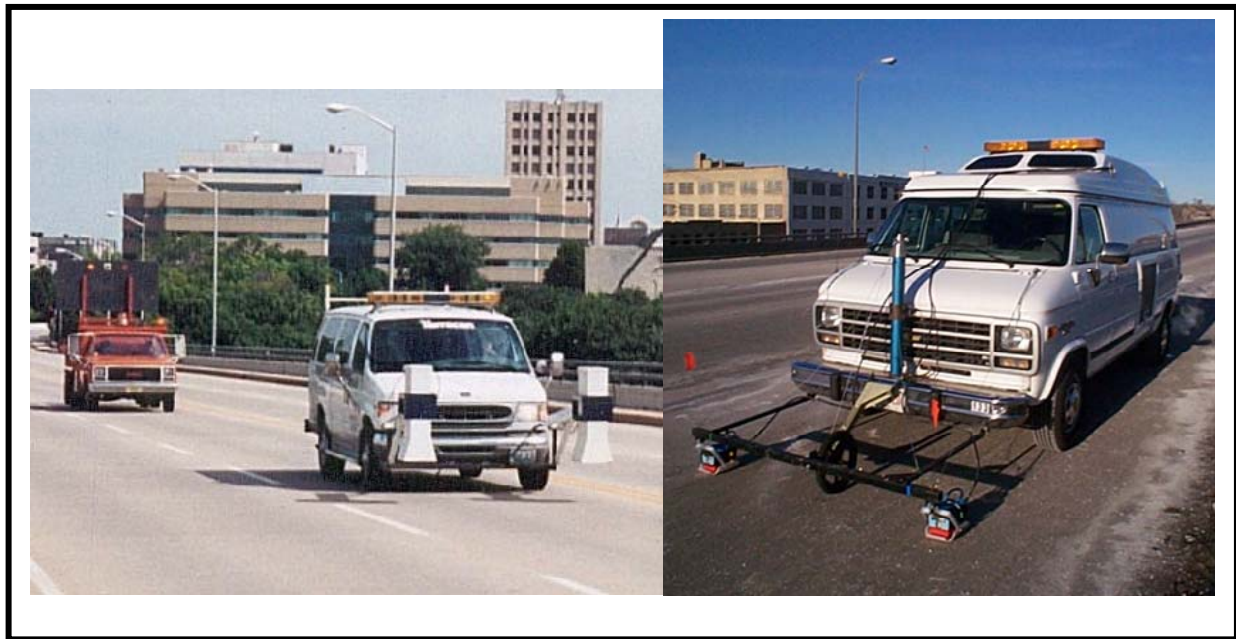
Figure 6:5-2: Horn Type (Left) and Contact Type (Right) Vehicle-Mounted Transducers
